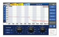
OTDR mode allows for measuring distance, loss, reflectivity, attenuation and accumulation loss on a fiber optical link.
