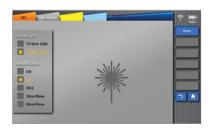
Invisiable light source (1310 or 1550ns) can provide the following types of light, including CW light, 1kHz light, 2kHz light, 1kHz blink light, 2kHz blink light.
